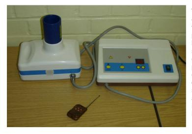
The operating potential and tube current are fixed and exposure times are selected on the control panel. Times can be selected between 0.1 and 9.9 seconds, in 0.1 second increments. X-ray exposures are triggered by either pressing an exposure button on the control panel or on the X-ray tube, or by using the remote exposure switch. The X-ray tube can be attached to a tripod if required but is intended to be used held in the hands.
