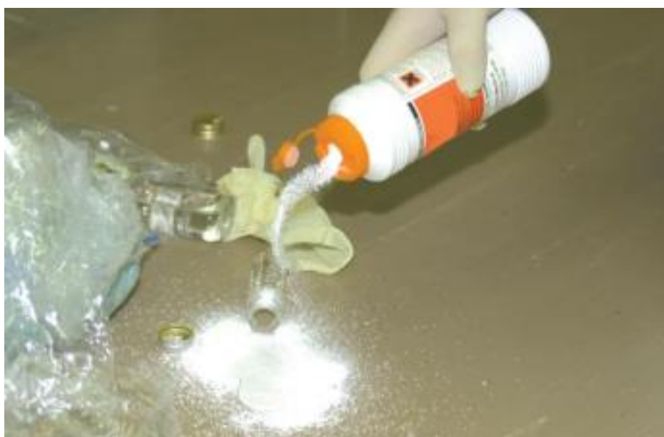
Figure 16 Clearing up a small liquid spill
