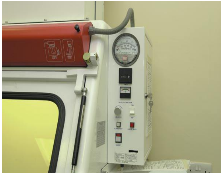
Figure 8 Alarms/indicators on safety cabinet
