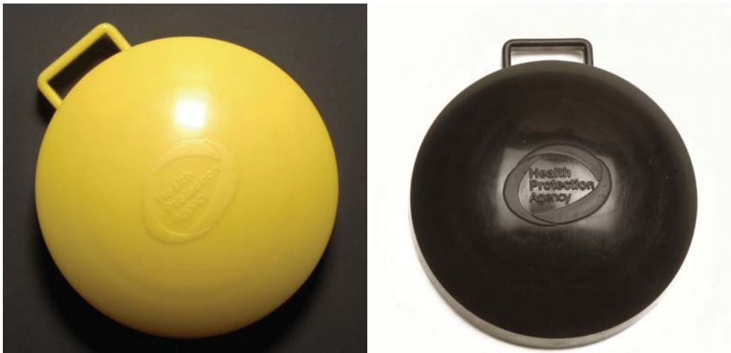
Figure A1. Old (yellow) and new (black) passive radon detectors.
