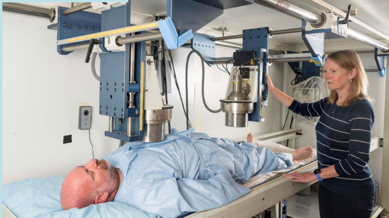
Picture of the UKSHA whole body monitor used to measure gamma emissions from the body to estimate internal dose
